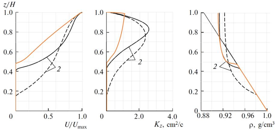
Fig. 1. Vertical distributions of the main flow characteristics for variant 2 at the time 240 s:  $e - \varepsilon$ -model (dashed line), improved model from work [2] (solid line), models 1,2 (yellow lines)
