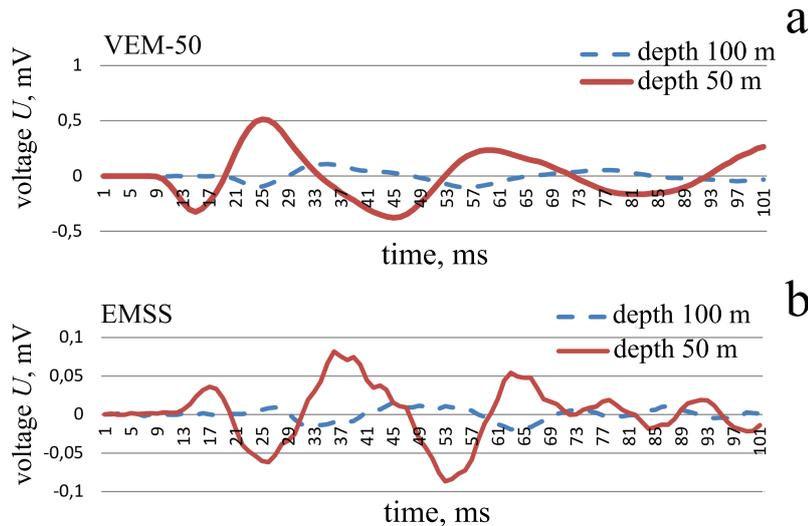
Fig. 4. The seismic signal recorded by the well acoustic sonde: a — from the VEM-50 seismic source; b — from the experimental model of the EMSS
